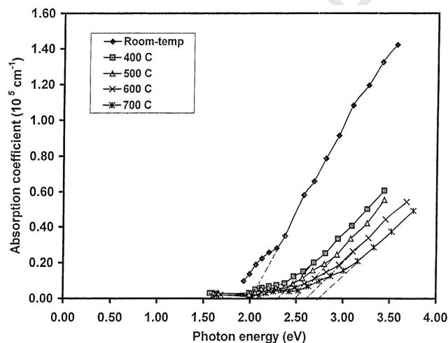
Fig. 2. Graphs of absorption coefficient ( $\alpha$ ) versus photon energy of SiC films, as-deposited and annealed in oxygen.
