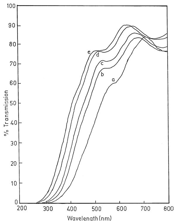
Fig. 1. Optical transmission characteristics of SiC films deposited at different temperatures, (a) as-deposited, annealed in oxygen at (b) 400 °C, (c) 500 °C, (d) 600 °C, (e) 700 °C.
