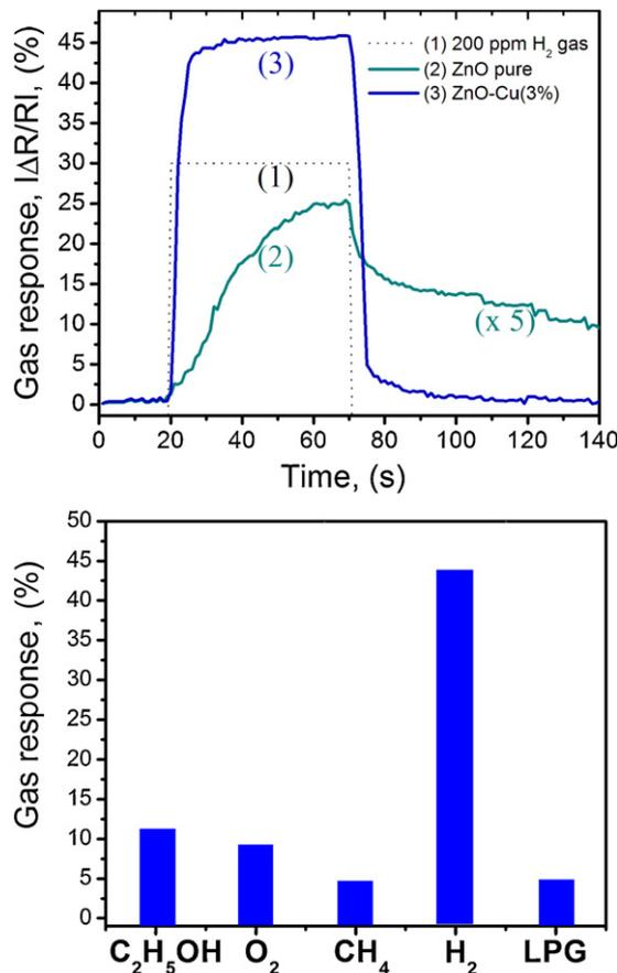
**Fig. 7.** (a) Room temperature relative response (multiplied by 5) of the conductometric single ZnO one-dimensional rod (curve 2) and single Cu-doped ZnO (curve 3) rod-based sensor structure fabricated by in situ lift-out technique in the FIB system to 200 ppm  $H_2$  gas (curve 1). (b) Gas response of a Cu-ZnO rod based sensor to different ambient of 200 ppm concentration.
