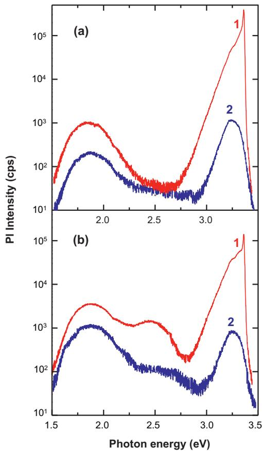
**Fig. 4.** PL spectra of: (a) 0.5% Cu-ZnO and (b) 3.0% Cu-ZnO rods measured at  $T = 10$  K (curve 1) and  $T = 300$  K (curve 2).
