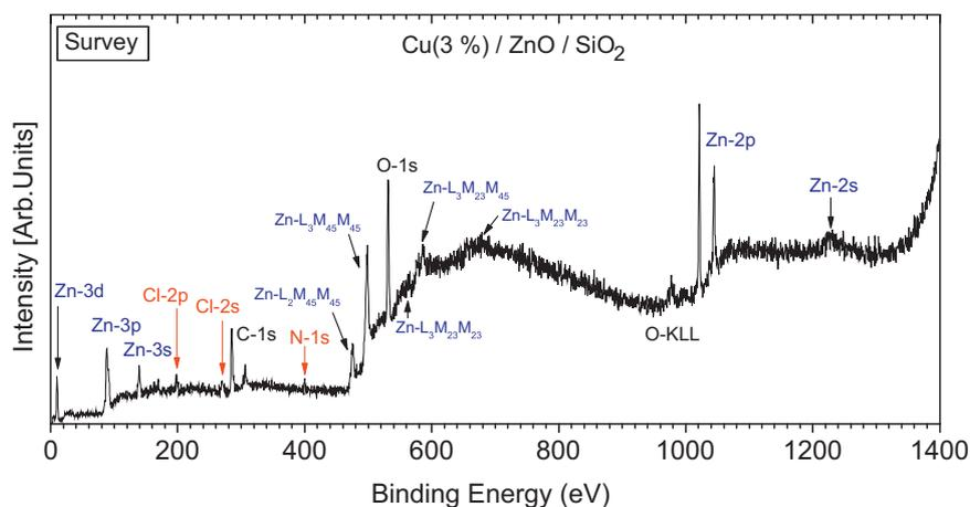
**Fig. 2.** Survey XPS spectra (Al  $K_{\alpha}$  = 1486.6 eV) corresponding to Cu-doped ZnO rods supported on  $\text{SiO}_2/\text{Si}(001)$ . In addition to Zn, other elements detected were O and adventitious C, Cl and N residues from the sample preparation method. The different photoelectron and Auger electron peaks observed for the latter elements are labeled in the graph.
