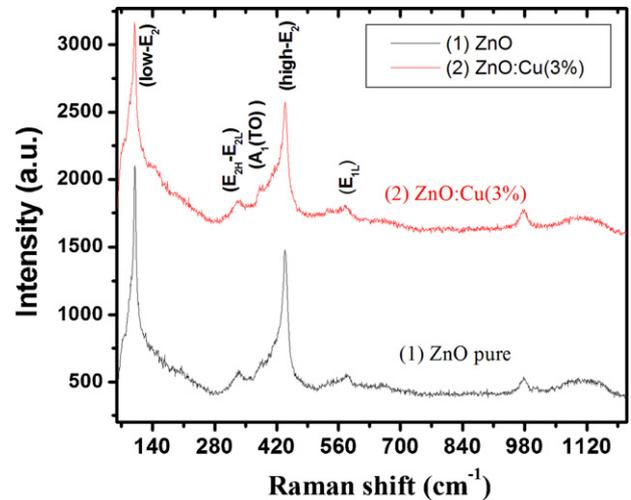
**Fig. 5.** Micro-Raman spectra of pure ZnO and Cu-doped ZnO on Si substrates.
