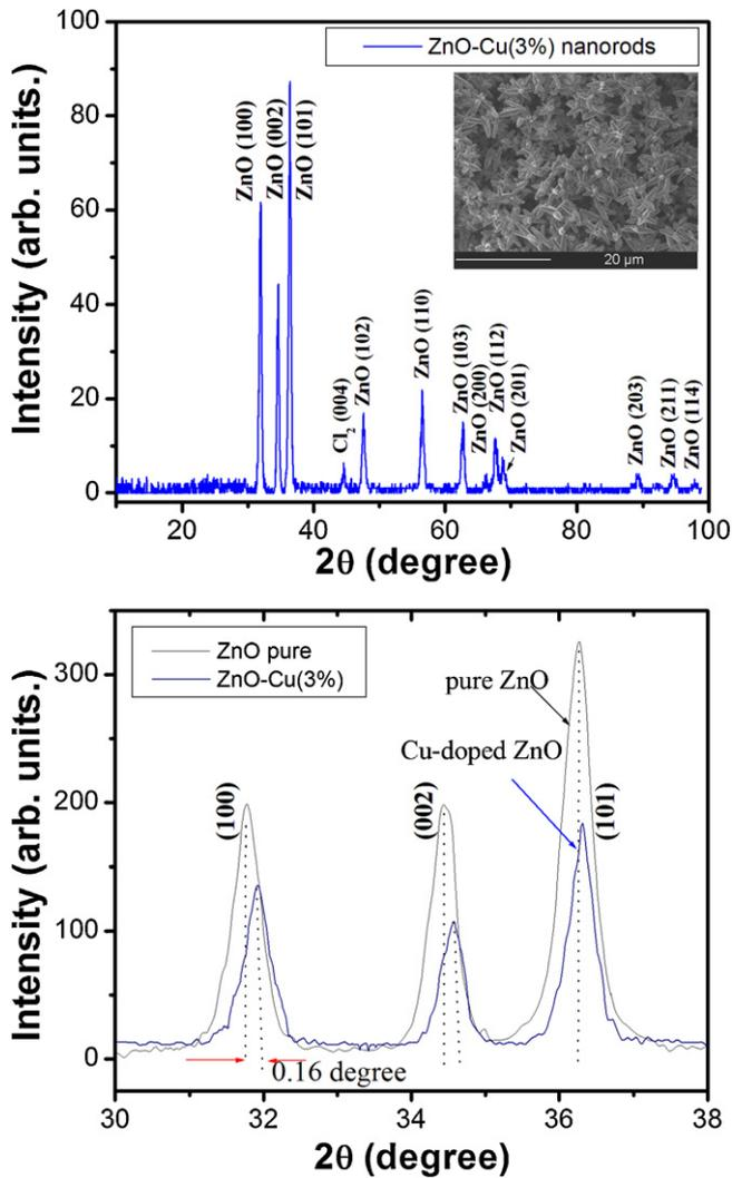
Fig. 1. (a) XRD patterns of the 3% Cu-doped ZnO nanorods on substrates. Insert shows an SEM image of 3% Cu-doped ZnO rods on SiO<sub>2</sub>/Si(001). (b) Comparison of the (100), (002) and (101) peaks taken for pure ZnO and 3% Cu-doped ZnO.
