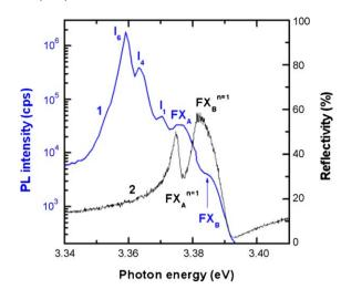
**Fig. 8.** The neutral donor- and free-exciton lines in the luminescence (1) and reflectivity (2) spectra of ZnO layers grown by CVD. T = 10 K.
