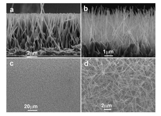
**Fig. 3.** SEM images of the cross-section of ZnO nanowire arrays with respect to the substrate position in the growth zone: (a) at the entrance of the growth zone (ratio O/Zn is larger), (b) at the exit of the growth zone (ratio O/Zn is smaller). Next are the SEM top-view images: (c) of the ZnO nanowires grown on ZnO/Si placed at the exit of zone (ratio O/Zn is smaller), (d) zoom in view image of the ZnO nanowires.
