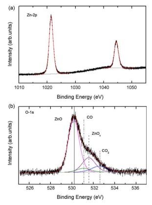
**Fig. 6.** XPS spectra (Al K $\alpha$  = 1486.6 eV) corresponding to the (a) Zn-2p and (b) O-1s core level regions of ZnO nanowires supported on SiO<sub>2</sub>/Si(0 0 1).
