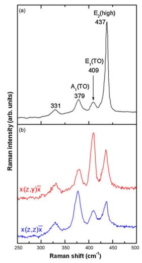
**Fig. 9.** Room temperature micro-Raman spectra of the ZnO nanowires: (a) non-polarized Raman spectrum measured in the quasi-backscattering geometry in the region of the TO phonons. (b) The polarized Raman spectra measured in-plane, i.e. from the edge of the sample (in the *x*-direction).
