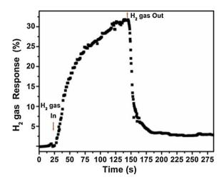
Fig. 11. Gas-response curve of the individual zinc oxide nanowire-based gas nanosensor under exposure to 100 ppm of  $H_2$  gas at room temperature.
