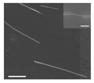
Fig. 10. Scanning electron micrograph of transferred ZnO nanowires. The insert shows device based on a single nanowire of 50 nm in diameter. Scale bars are 2  $\mu$ m.
