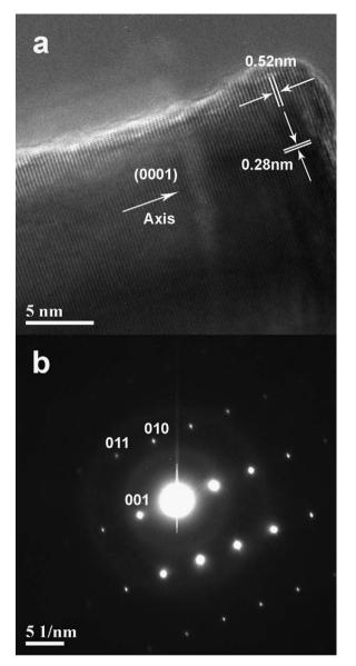
**Fig. 4.** (a) HRTEM image of ZnO nanowire grown by CVD method and (b) its corresponding selected area electron diffraction SAED pattern.
