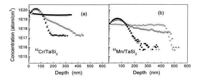
Figure 3. SIMS depth profiles of (a)  ${}^{52}$ Cr (120 keV, 1.1E15 ions/cm<sup>2</sup>) and (b)  ${}^{55}$ Mn (150 keV, 1.1E14 ions/cm<sup>2</sup>). (• As-implanted,  $\circ 300^{\circ}$ C,  $\blacktriangle 500^{\circ}$ C,  $\bigtriangleup 700^{\circ}$ C,  $\times 900^{\circ}$ C,  $\blacksquare 1000^{\circ}$ C).
