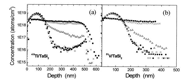
Figure 2. SIMS depth profiles of : (a)  ${}^{39}$ Ti (150 keV, 1E14 ions/cm<sup>2</sup>) and (b)  ${}^{51}$ V (150 keV, 1E14 ions/cm<sup>2</sup>). (• As-implanted,  $\circ$  300°C,  $\blacktriangle$  500°C,  $\triangle$  700°C,  $\times$  900°C,  $\blacksquare$  1000°C).
