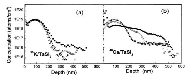
Figure 1. SIMS depth profiles of : (a) <sup>39</sup>K (150 keV, 1E14 ions/cm<sup>2</sup>) and (b) <sup>40</sup>Ca (150 keV, 1E14 ions/cm<sup>2</sup>). (• As-implanted,  $\Delta$  700°C, × 900°C, = 1000°C).
